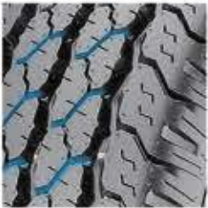
Extra-wide zigzag grooves deliver enhanced wet traction and exceptional low speed traction.
