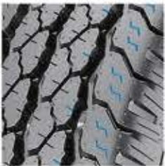
Full-depth microspikes Improve heat dissipation and traction.
